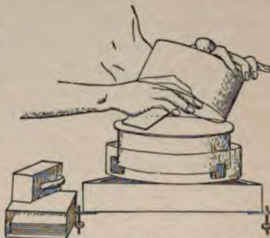
FIG. 21.—Koch's levelling apparatus. Hands shown in second position just as the plate is lowered on to the ground-glass surface. By executing the transference of the plate from the box in this way, the surface which was undermost in the latter is uppermost in the leveller, and thus never meets a current of air which might contaminate it.
